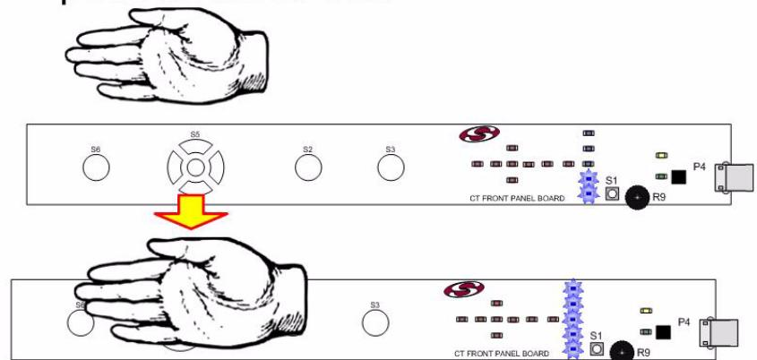
**5** Press the Sx capacitive sensing buttons on the board. Each will light a corresponding red LED when firmware senses a finger's presence.
