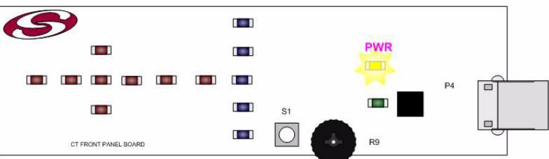
**4** Move a hand in close proximity to the board. This causes the array of blue LEDs to light up as the hand approaches. Adjust proximity sensitivity by rotating the potentiometer R9.
