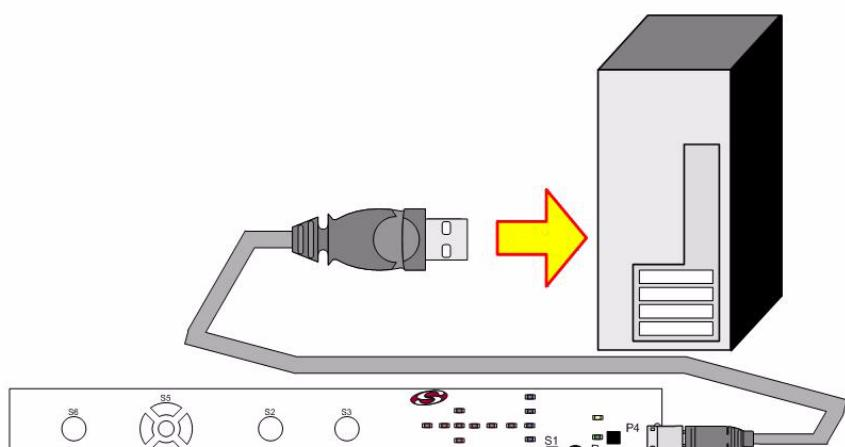
**3** Wait for enumeration to complete. Watch for the LED labeled PWR to turn on.
