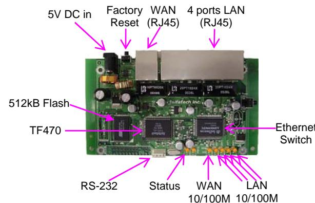
5V DC power (not included) is supplied through the power connector with positive polarity in the middle. Factory reset button is provided for reset to factory default setting.
