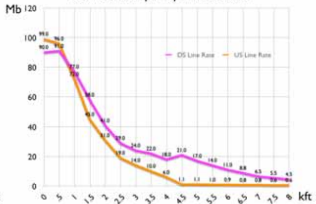
26 AWG, Band plan symmetric ISDN
